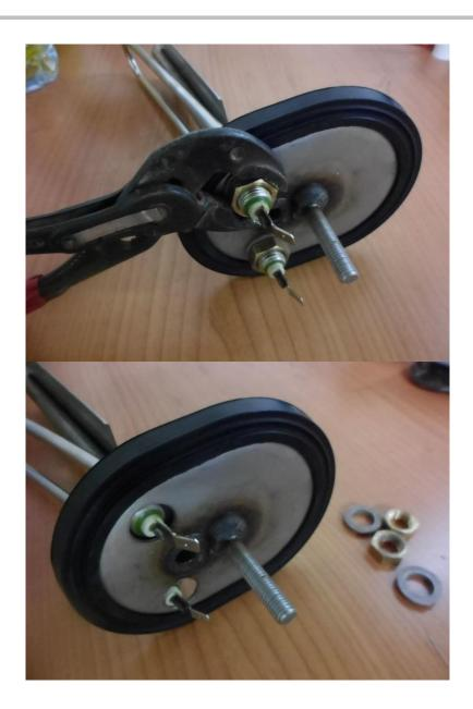
Remove the nuts holding the heating element
