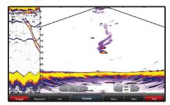
Shows real-time moving sonar images of small baitfish and large target fish swimming below your boat and pinpoints their distance left or right and their depths.
