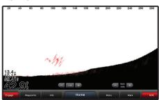
To help give you time to avoid collisions with submerged obstacles, FrontVü shows underwater obstructions within a 300' range as you approach them in real time<sup>1</sup>.
