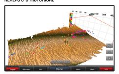
Scrolls through sonar data as the boat moves to show the history of the entire water column from the bottom to the surface and all of the fish in between.
