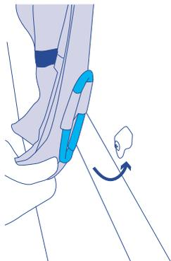
6 The elastic loops hold the bag securely in place and are tagged to assist clipping them on and off.
