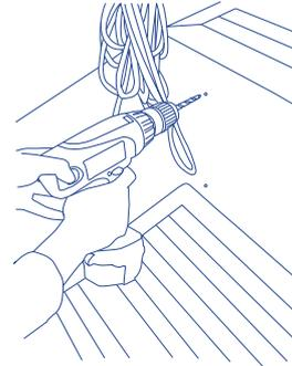
3 Screw the small white Blue Performance hooks in place, using the countersunk screws provided.
