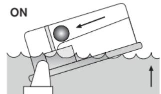
Water raises switch, ball rolls back, switch snaps on.
