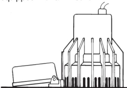
AS888 should always be installed in parallel to the keel with the floating body directed aft. Never install AS888 at a level lower than the inlet of the bilge pump.
