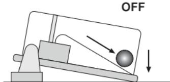
Ball at rest, switch in off mode.
