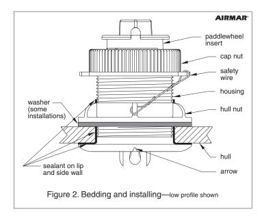
2. From inside the hull, slide any washer(s) onto the housing.
