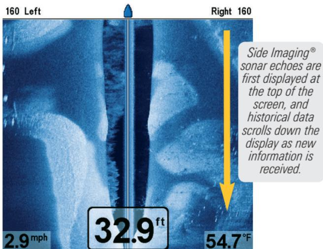
The main benefit of Side Imaging<sup>®</sup> sonar to anglers is that it provides an overall survey of a large area of water. This gives you a better understanding of the bottom topography and how structure is oriented for more efficient fishing.
