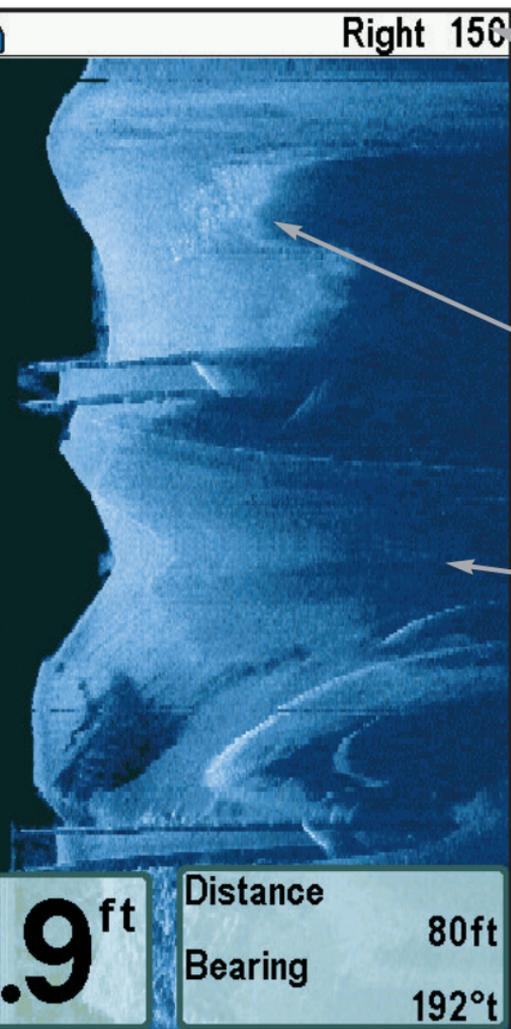
**Side Imaging® Range** - Images shown on the right side of the screen are located on the right side of your boat, and images shown on the left side of the screen are located on the left side of your boat. In this illustration, the sonar is pinging 150 feet on each side.
