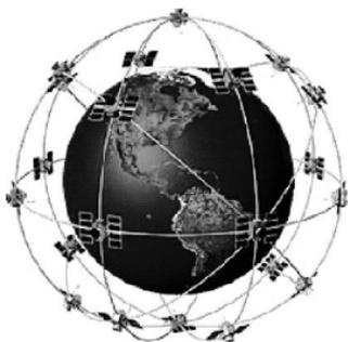
GPS uses a constellation of satellites that continually send radio signals to the earth. The GPS receiver on your boat receives signals from satellites that are visible to it. Based on time differences between each received signal, the GPS receiver determines its distance to each satellite. With distances known, the GPS receiver mathematically triangulates its own position. With 5 updates per second, the GPS receiver then calculates its velocity and bearing.
