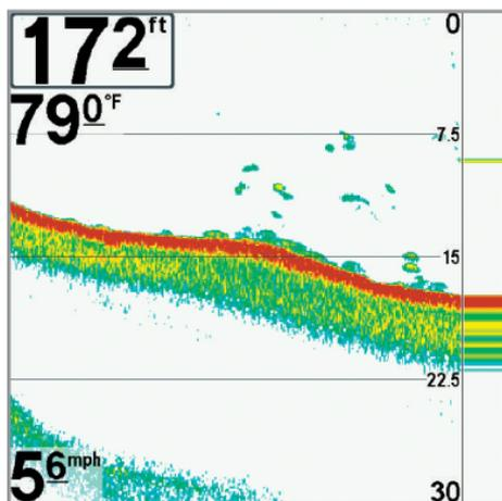
**Structure ID**<sup>®</sup> represents weak returns in blue and strong returns in red when Sonar Colors is set to Original. If the Sonar Colors palette is changed, the Structure ID<sup>®</sup> will display the strongest return as specified by the palette. See *Sonar Menu Tab: Sonar Colors* for more information.
