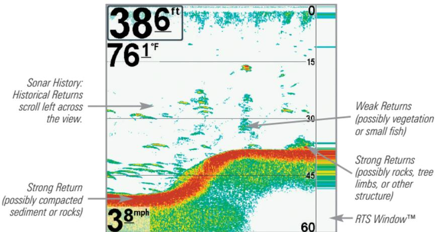
Use **Bottom View** to select the method used to represent bottom and structure on the display. See *Sonar Menu Tab* to set the Bottom View.
