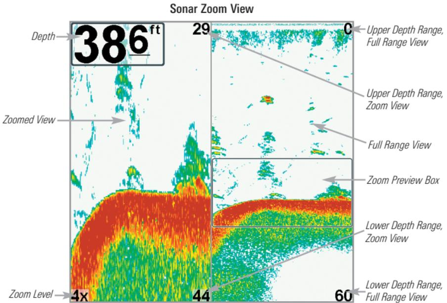
*Digital depth is displayed in the upper left hand corner. The digital readouts in the Sonar Zoom View cannot be customized; therefore, information such as water temperature and voltage are unavailable in the Sonar Zoom View.*
