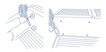
5 The back of each product has loops in each corner. Hang the top two cord loops over the hooks and stretch the two bottom elastic loops over the lower hooks.
