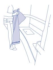
3 Choose a hole in the webbing closest to the front edge of the seat. Fix 5 x screw throught the webbing.
