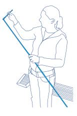
4 Tension the batten and force the tip in the corner pocket.
