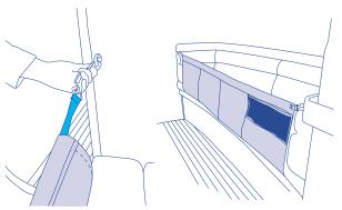
2 Place the bunknet with silver side up. Check if final height of the bunknet is ok.
