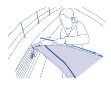
6 Fix its position using the corner cords attached to the railing.
