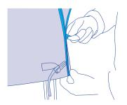
4 Define cover length to fit your boom with the separate flap at the rear. Adjust double layer of the flap and fix it with Velcro.
