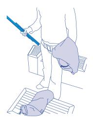
3 Guide the battens through loops and seat in each corner. Make sure the battens are crossed.
