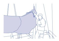
3 Fix the cover around the mast with the Velcro straps. Fasten with the buckle.
